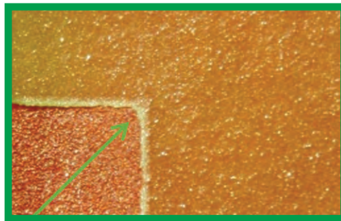
200°C for 2000 Hours; No Cracking on Copper or Laminate
