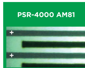
Insulation resistance: 3.2E12Ω
