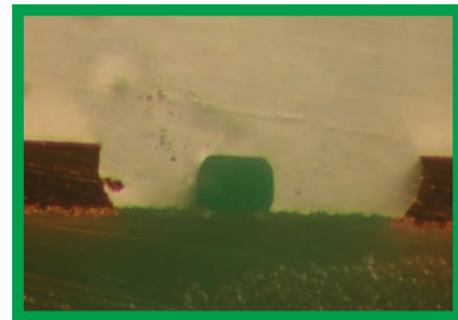
PSR-4000 BW01DI 2 Mil Dam Exposed at 80 mJ
