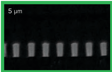
Cross Section View (L/S = 2 \mu m / 2 \mu m) 130°C, 85% RH, 5V
